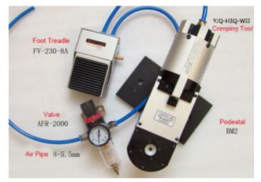
2. Adapts HD2-C001 Customized positioner. It contain a dials which has 8 selections to adjust the working diameters of the 4 indenters. (check the left table)
