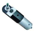
3. Crimping instruction: firstly insert the contact and wire, supply the air by foot treadle or manual button, release the foot treadle or manual button after the crimping complete. Takeout the contact when the indenter back to the original position.
